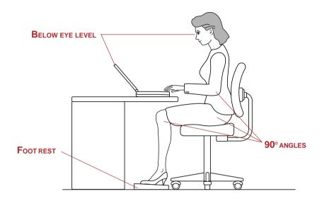
Figure 3-1 Posture and positioning of the computer
